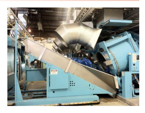
Minimize the accumulation of Soiled Linen in the washroom and sorting areas. Soiled linen is stored in the hopper or chute, ready for immediate loading to start the next wash cycle.
